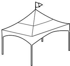
Aluminum frame and canopy weight varies by configuration and has an eave height of 8'. Comes with carry bag, steel stakes and guy ropes.
